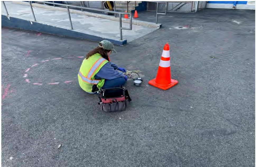
Photograph 8: View of soil vapor purging and sampling activities at boring B38/SV2
