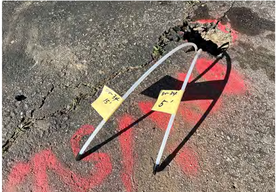
Photograph 9: View of 5 and 15 foot soil vapor probes at boring location B34/SV5, prior to patching.
